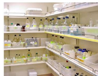
Chemical Shelving with Lips to Prevent Falling
