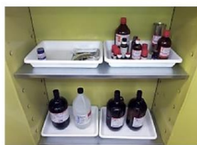
Chemicals Stored in Secondary Containers
