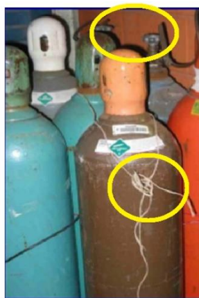
Cylinders Tied with Rope Cylinders without Cap ❌
